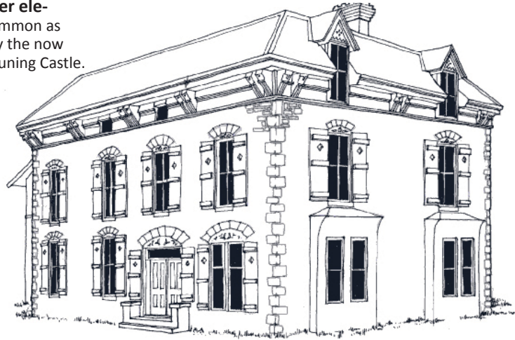
Overall massing can be a simple symmetrical "classical" block or an asymmetrical romantic composition.
