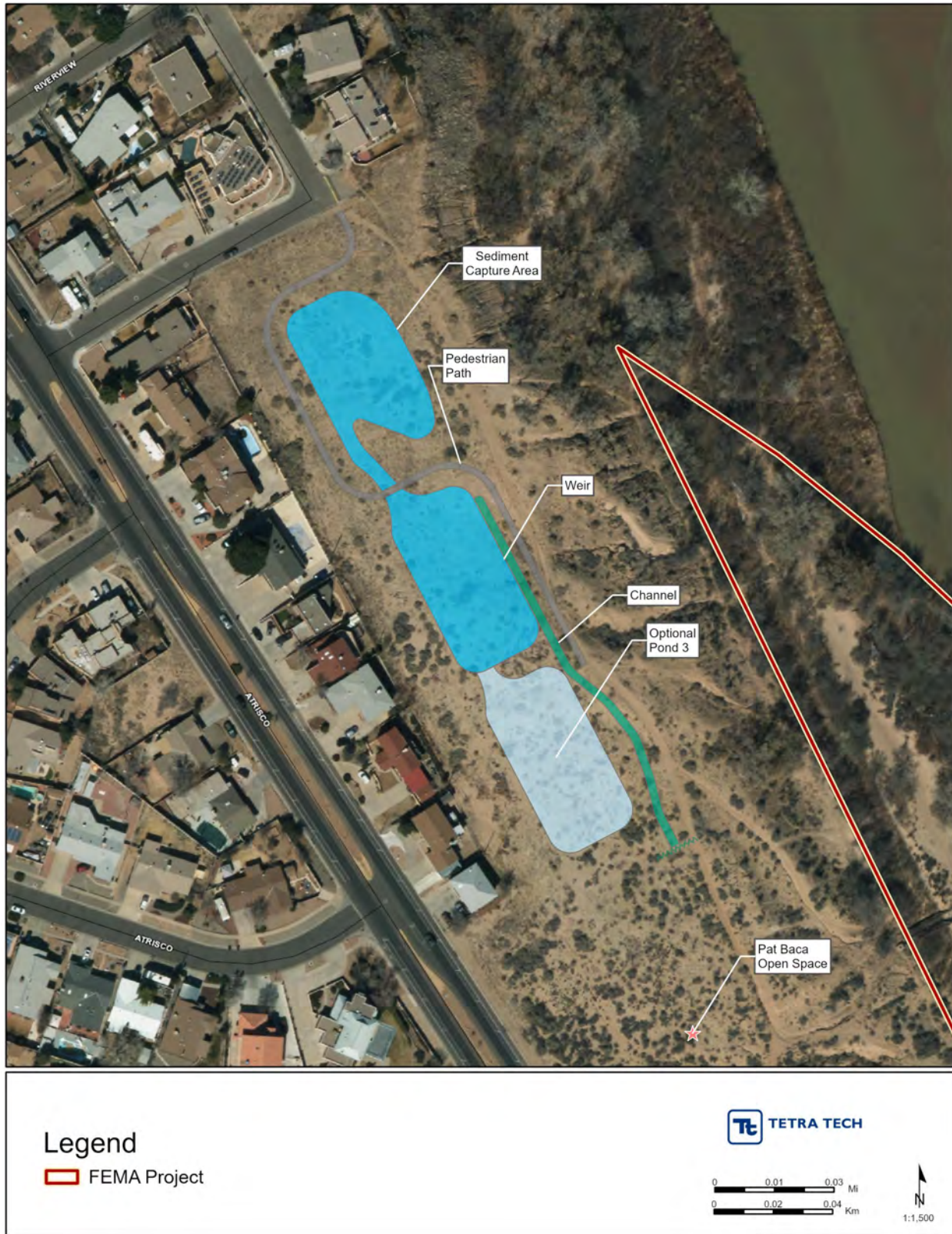
Figure 18. Outfall Restoration Alternatives
