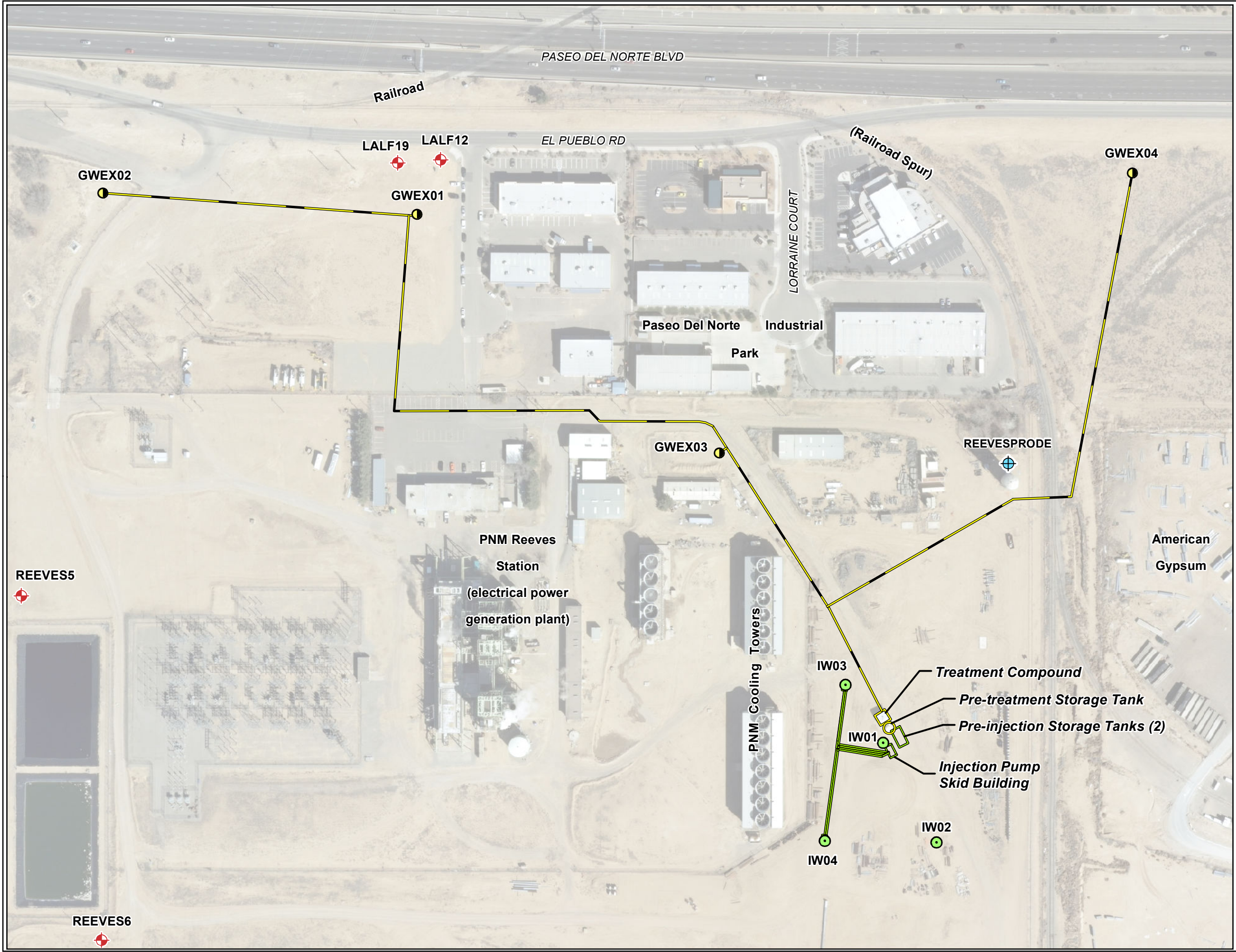
Figure 4 Groundwater Pump-and-Treat System Layout Map COA - Los Angeles Landfill Landfill Management Plan
