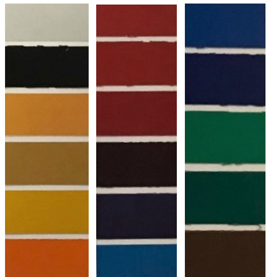
Examples of the variety of colors of high visibility reflective sheeting; the sheeting can be used on sign faces, posts, or lettering to match or complement sign materials.
