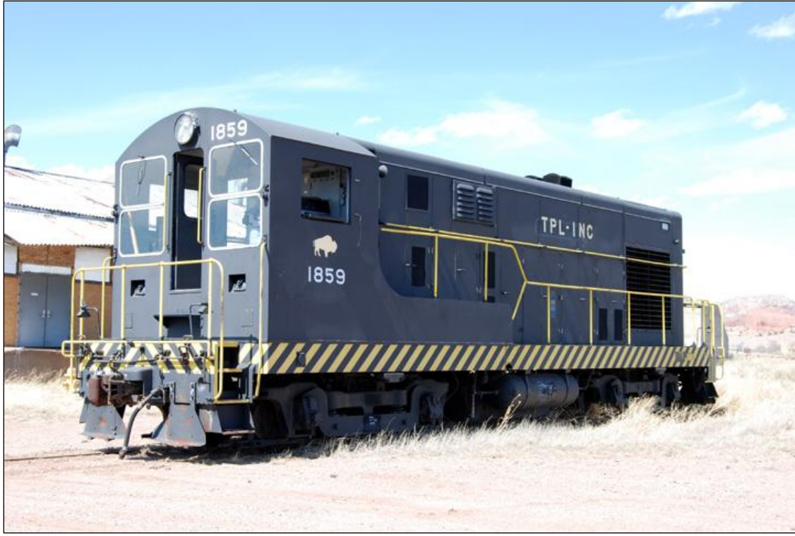
Figure 7 Donated Operating 1953 Fairbanks Morse 12-44 Diesel Switcher Locomotive Waiting for Shipment from Ft. Wingate, NM to WHEELS
