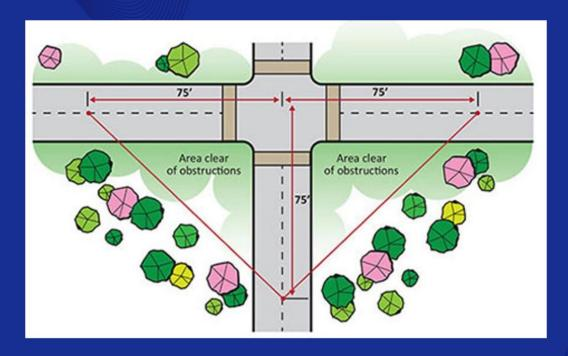
The clear sight triangle is the area between curb lines of an intersection and line connecting points at a specific distance from the corner of the intersection and such corner is determined by projecting the curb lines out to a specific point
